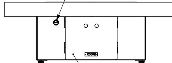
Access Door for tank or gas connection
